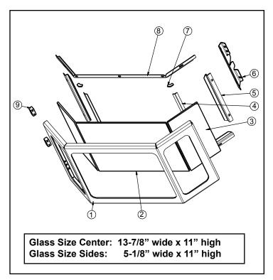
Figure 37.1 - Door, Face, Glass & Door Latch Assembly
